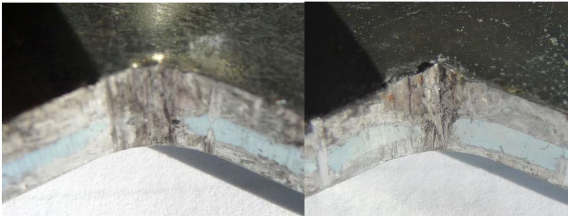
**Figure 12** *The upper and lower bearing surfaces of the hook. Note the triangular groove in the inner edge of the lower hook bearing surface.*
