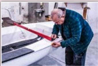
Measuring depth of cockpit at Station 2
