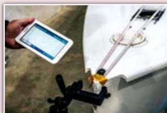
Using a tablet to time oscillations
