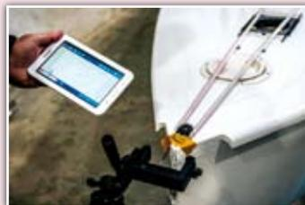
Using a tablet to time oscillations
