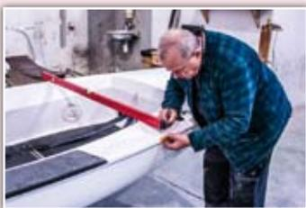
Measuring depth of cockpit at Station 2
